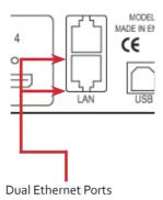
Connect the Fx4-SDI to a network using the top LAN connector then open Wall Designer and create your display layout. At the point where you associate the virtual device with a physical device the list will display all Fx4-SDI's currently connected to the network either directly or daisy chained.
