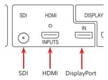
Connect your input source to one of the 3 input connectors on the rear of the Fx4-SDI. You can connect up to 3 input sources,  $1 \times SDI$ ,  $1 \times HDMI$  and  $1 \times DisplayPort$ .
