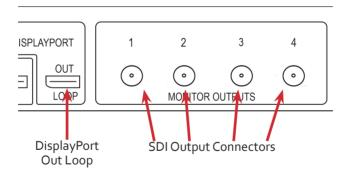
Connect the SDI cables to the SDI output connectors on the rear of the Fx4-SDI, you can connect up to 4 devices to a single Fx4-SDI unit. Ensure the cables are inserted correctly, rotated and locked.
