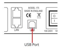
When the Fx4-SDI has booted, connect it to your PC using the USB cable provided. The Fx4-SDI unit is a plug and play device, Wall Designer will detect it when the layouts are configured.
