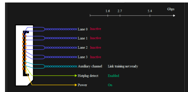
Status information of the disconnected port
